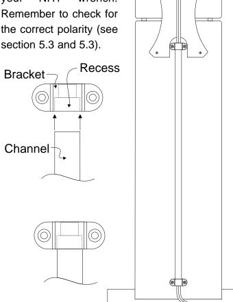
Slip the channel over the speaker wire. The brackets are recessed on one side to accept the
